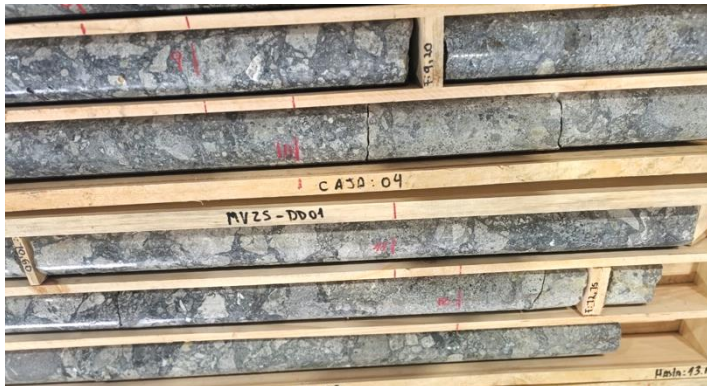
MV25-DD01: Hydrothermal Breccia, Dacite porphyry fragments in dark-gray hydrothermal matrix. 9.2-meter depth block at photo top.
